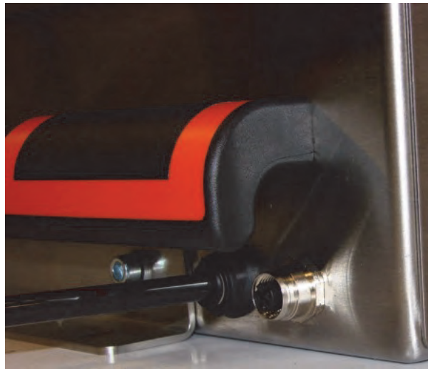
Figure 2-6. Air Line Attached to Pneumatic Connector
